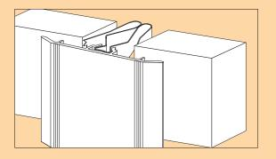
4. Firmly squeeze the top of the spring clip and slide down the channel to desired location.
