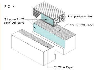
Installation of Compression Seal without Vacuum Pump.
