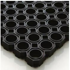
Material : solid rubber, abrasionproof, weatherproof Surface : honeycomb : knops, 3/25" (3mm) - to allow drainage Bottom Thickness : 9/10" (23mm) Color : black : approx. 21 lbs/sqm (9.5 kg/sqm) Weight Properties : high cleaning effect, dimensional stability, robust, easy to clean particularly suitable for areas subject to wetness, snow and sand.
