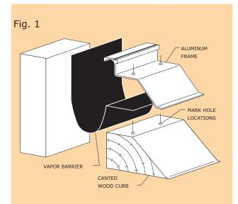
1. Install the architectural joint system on a level surface. To ensure + / - 50% movement, top of canted wood curb must be  $1-\frac{1}{2}$ " (38mm) -  $1-\frac{3}{4}$ " (44mm) wide.
