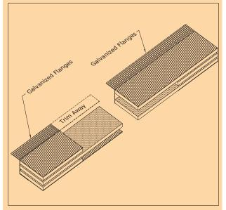
The splicing of the interior insulation materials, screen and interleafed metallic foils are to be performed in the same manner as the rilled version of ZFS.
